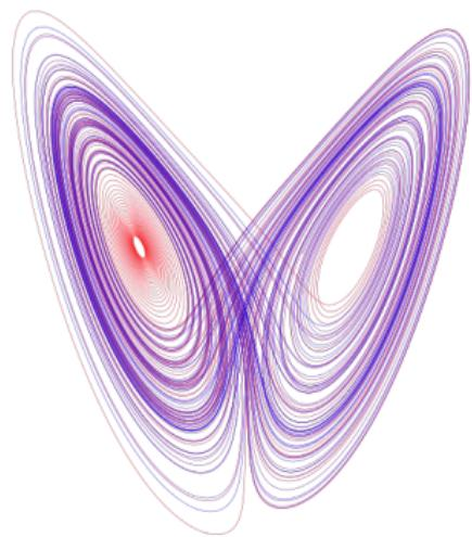
$$\begin{aligned}\dot{x} &= 10(y - z) \\ \dot{y} &= x(28 - z) - y \\ \dot{z} &= xy - \frac{8}{3}z\end{aligned}$$
